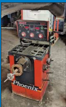
Coats Model 1001R Tire Balancer
