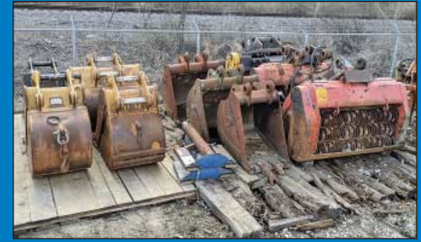
(3) 70" Wide Hydraulic Excavator Screening / Padding Buckets by Allu & Nye
