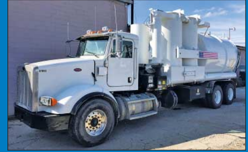
2013 Peterbilt Chassis w/ Super Products Model 6227 Super Sucker Vacuum System
